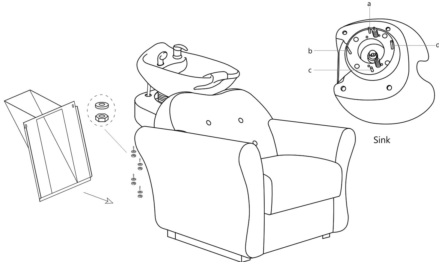
Undo the access panel by twisting clockwise then using the 4\* 14mm washers & gaskets provided fasten the sink to the base.
