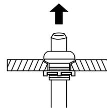
Place the sprayer hose from underneath through the sprayer head holder and fasten the sprayer head to the sprayer hose.
