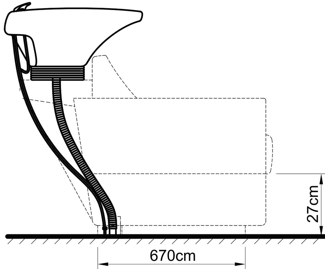
Secure the backwash on the floor by the provided floor anchors.
