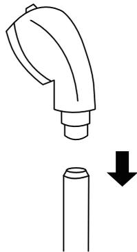
Unscrew the sprayer head from the sprayer hose.
