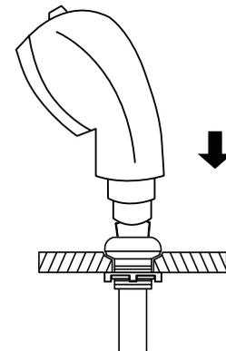
Place the sprayer hose from underneath through the sprayer head holder and fasten the sprayer head to the sprayer hose.
