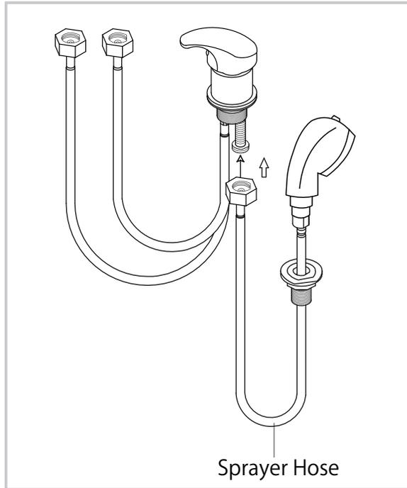
Connect to sprayer hose to the tap shown in the diagram.
