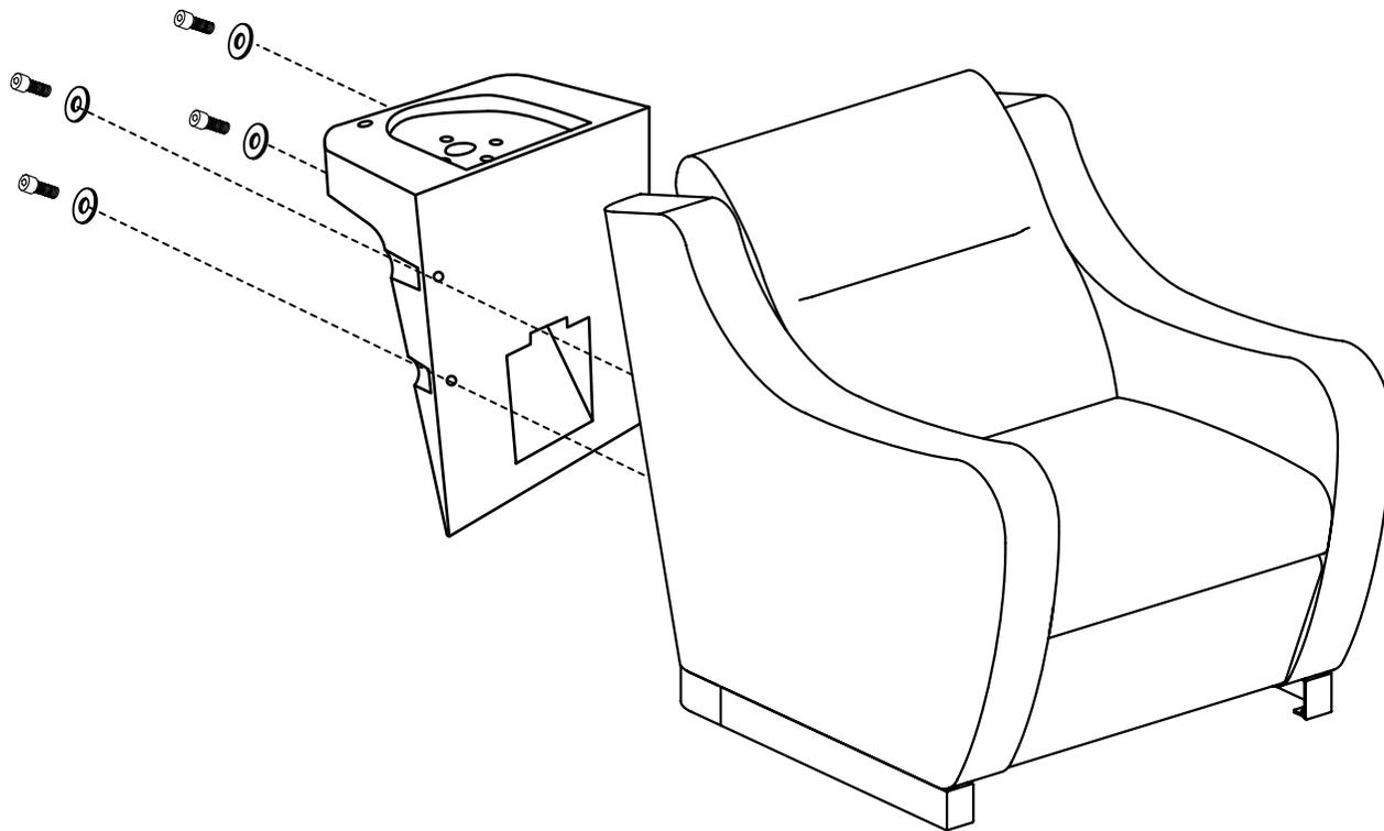
Secure the Cover on the back of the backwash.
