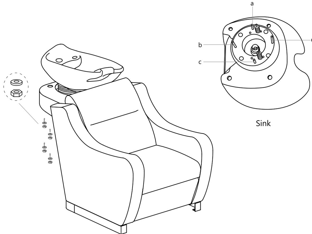
Undo the access panel by twisting clockwise then using the 4\* 14mm washers & gaskets provided fasten the sink to the base.
