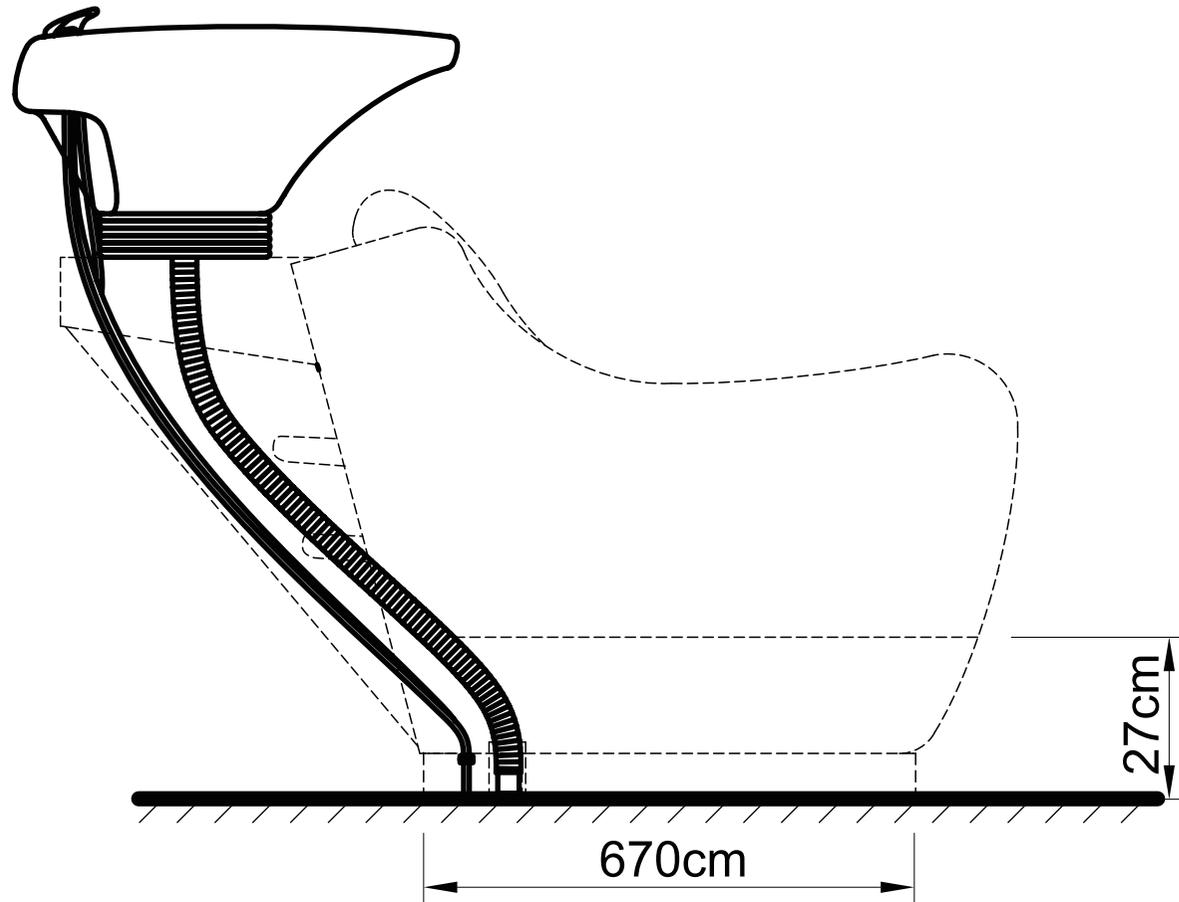
Secure the backwash on the floor by the provided floor anchors.
